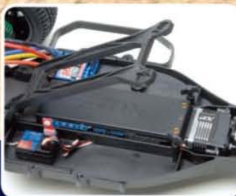
Hinged battery hold-down strap for quick and easy access
