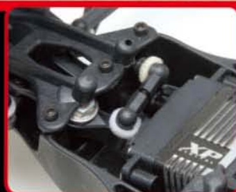
Angled bellcrank "coplanar" steering with integral servo saver
