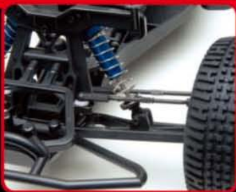
Rugged steel turnbuckles and blue aluminum shock bodies
