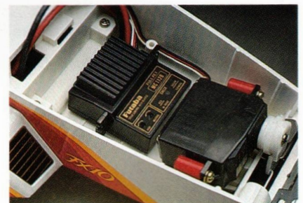
The MC112B is ideal for offroad cars like our FX10. It features MOS/FET design with reverse and installs conveniently in place of the throttle servo.
