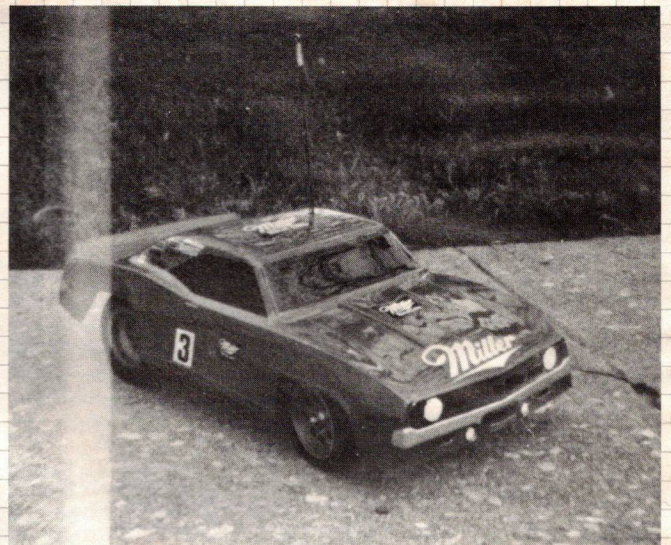
This '67 Camaro body masks a modified Fox underneath. It is the work of Greg Matuson, of Coatesville, Pennsylvania who says his car has 14 ball bearings and a Trinity offroad stock motor.
