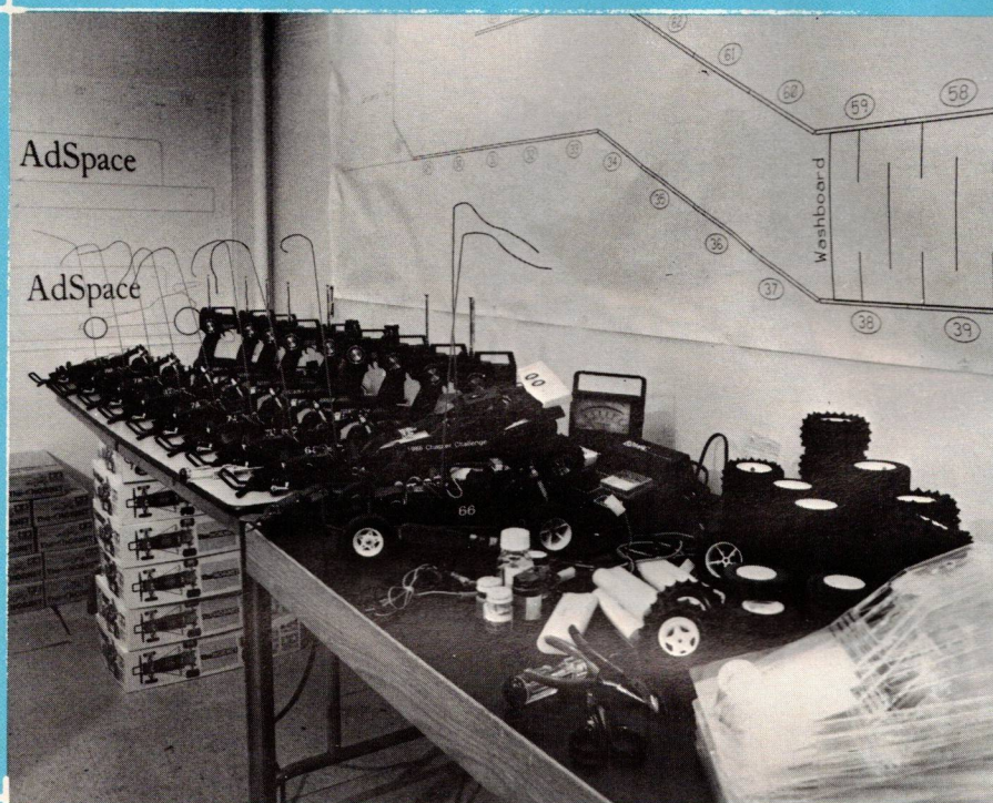
The first two Hornet chassis were assembled individually to check for bugs (there weren't any), then the other eight racers were mass-produced.
