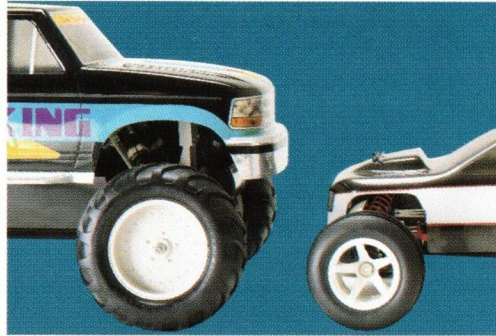
World Scale trucks like the Baja King or Thunder King (shown here) are longer and wider, with 50% more mass than 1/10 scale.
