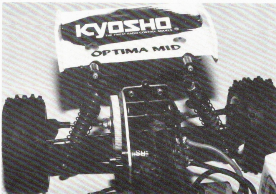
Location of the new upper rear shock holes when the output shaft has been modified.
